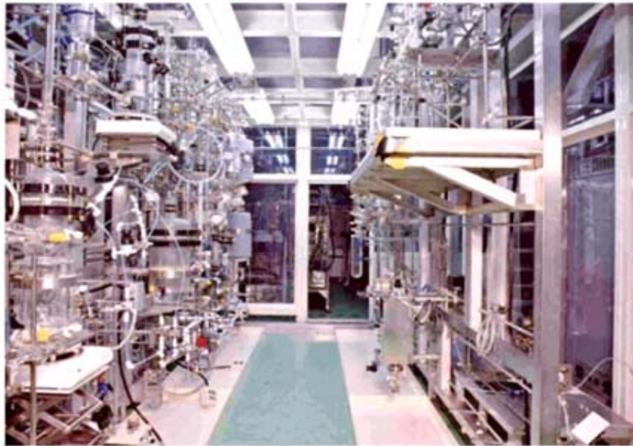
Photo: Continuous Hydrogen Production Test Apparatus (Near left: Bunsen reaction step equipment. Far left: Sulfuric acid decomposition step equipment. Far right: Hydroiodic acid evaporation/decomposition step equipment.)
