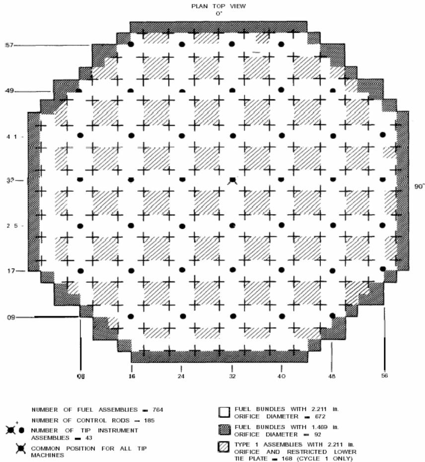
**Figure 3.6:** Core orificing and TIP system arrangement
