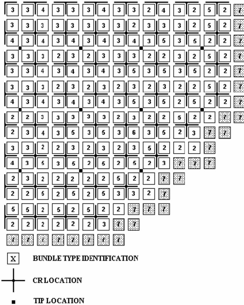
Figure 3.5: Assembly type identification, TIP and Control rod location
