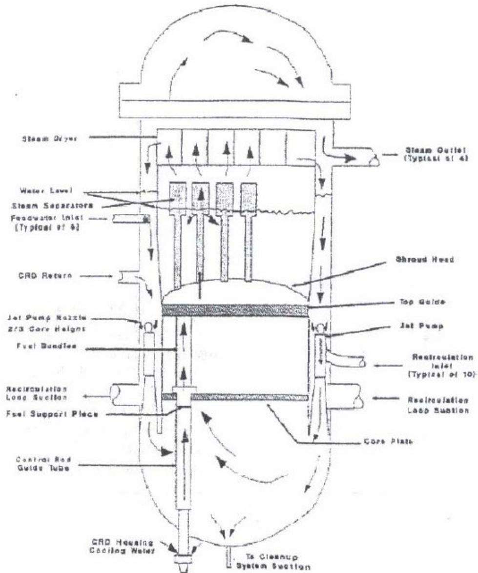
REACTOR VESSEL AND INTERNALS
