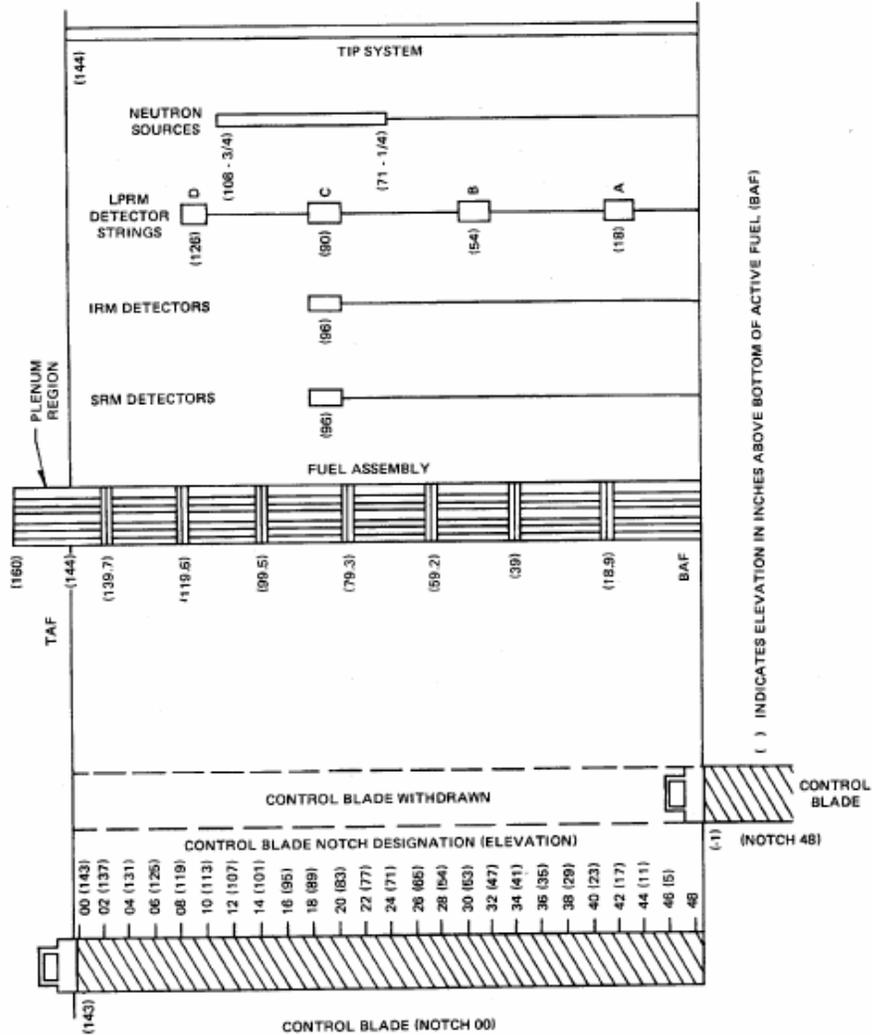
Figure 3.7: Elevation of core components
