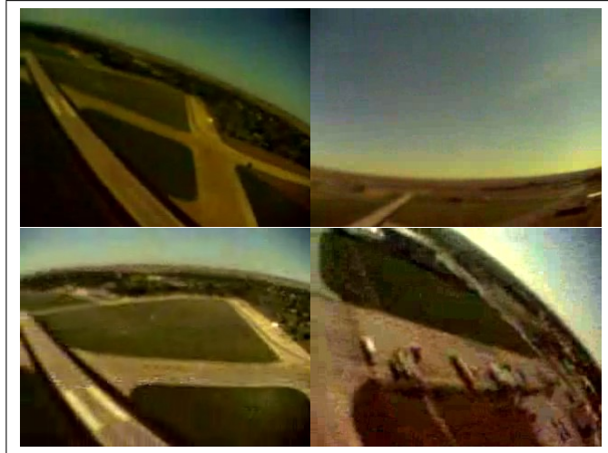
Figure 6-9: Radial distortion in video frames
