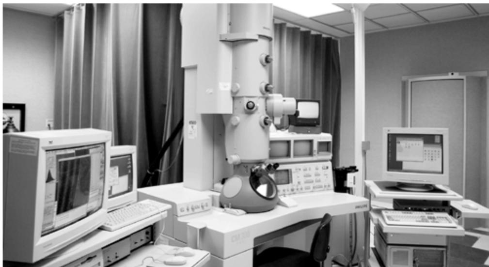
Metallurgists are probing the microstructure of actinides with a transmission electron microscope capable of near-atomic resolution.
